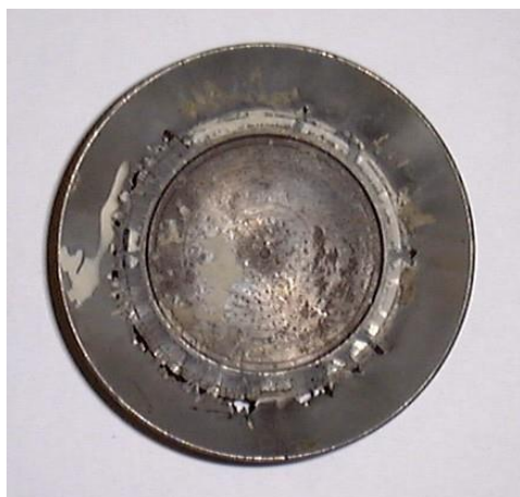
Figure 17.3.1-1: Symptom 1 – Disc worn out due to permanent leakage
